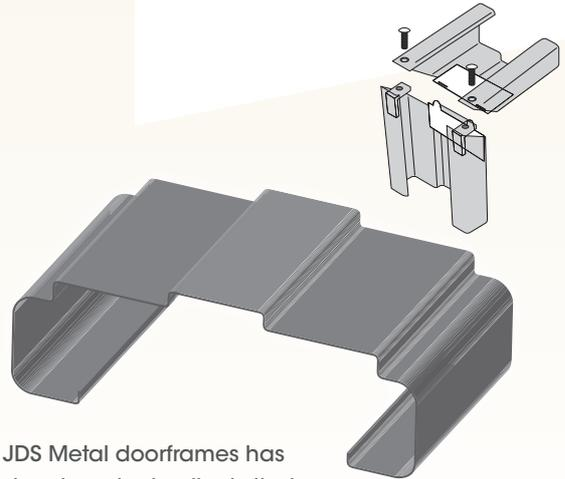
The JDS Deluxe Knockdown is used for stud frame construction. JDS Metal doorframes has decided to manufacture the Deluxe profile in the knockdown system to cater to clients that are renovating or adding an extension to their property, using stud frame construction and would like to keep the same profile as existing doorframes. The patented knockdown design system allows the mitre corners to be adjusted, resulting in an accurate and neat mitre joint.
