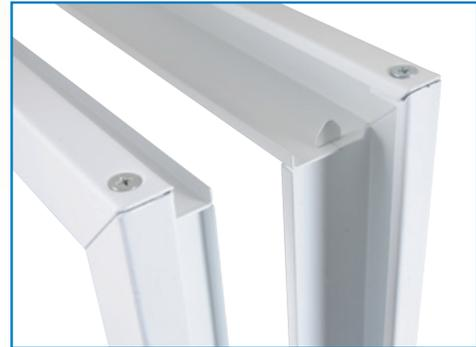
JDS Cavity Slider Metal Doorframes are manufactured from 1.0mm Zincanneal with a standard 114mm back opening to suit 90mm stud work with 10mm plasterboard either side. Cavity Slider units are available in two door heights of 2040 or 2340mm in various standard widths.
